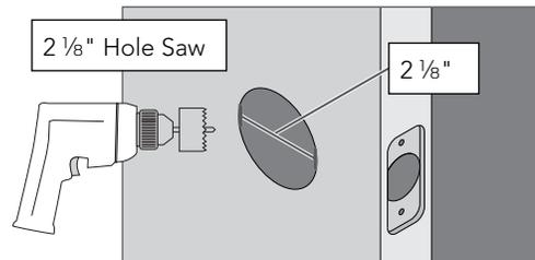
3c If necessary, enlarge hole in door edge.
