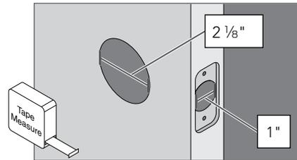
3b If necessary, enlarge hole in door face.
