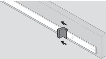
**F** Slide door stop so it touches the hanger. Tighten the set screws to secure it in place.
