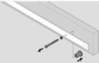
**C** Slide the door stop onto the track, past the hole where the fasteners were removed.
